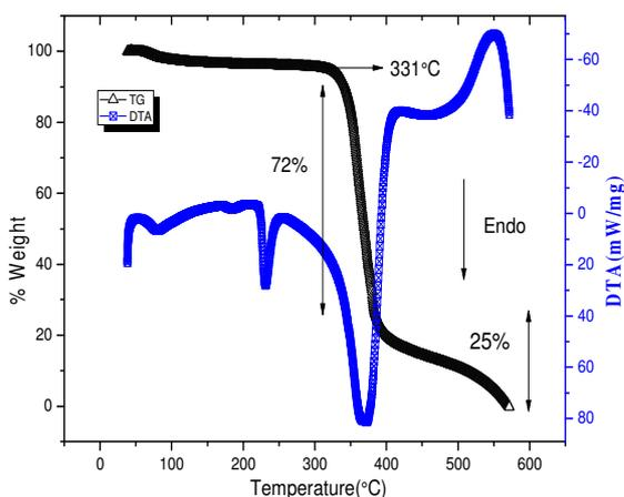
Figure 2. TG-DTA curve of IMT
