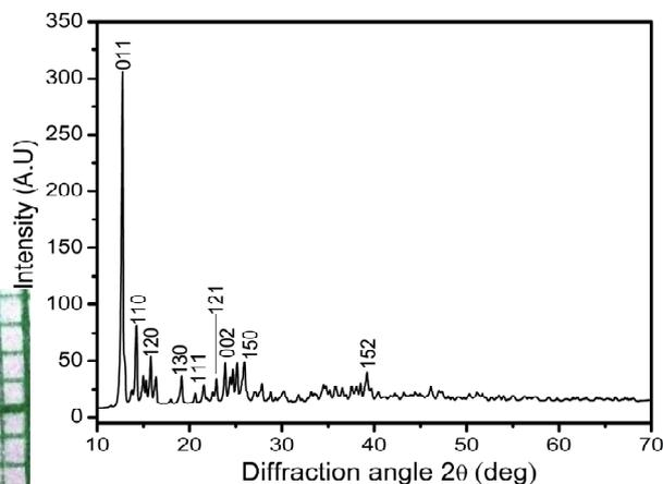
FIGURE.3 Powder X-ray diffraction pattern of 2-APC crystalline sample
