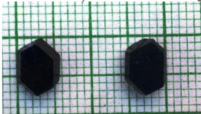
FIGURE.2: Photograph of as-grown 2-APC single crystals
