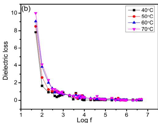
**FIGURE. 5(a)** Plot of dielectric constant vs. Log f and **(b)** Plot of dielectric loss vs. Log f of 2-APC crystalline material
