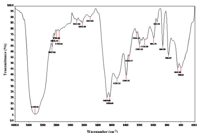
FIGURE 4 FT-IR spectrum of 2-APC crystalline sample
