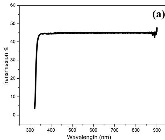
FIGURE.5 (a) UV-Visible transmittance spectrum and (b) Photoluminescence spectrum of 2-APC crystal
