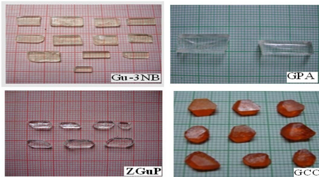
Fig. 1.1(a) Seed crystals of Gu-3NB, GPA, ZGuP and GCC grown by slow evaporation technique
