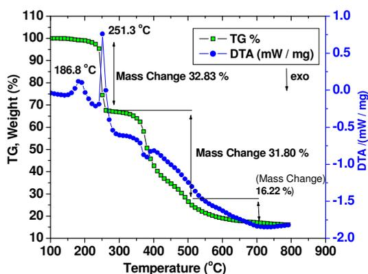
Fig. 3.3 TG-DTA thermogram of Gu-3NB and GPA
