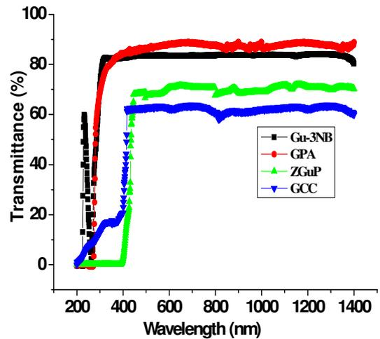
Fig. 3.1 Transmittance spectra of grown crystals
