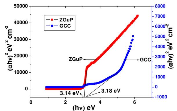
Fig. 3.2 plot of  $(\alpha hv)^2$  vs  $h\nu$  for grown crystals
