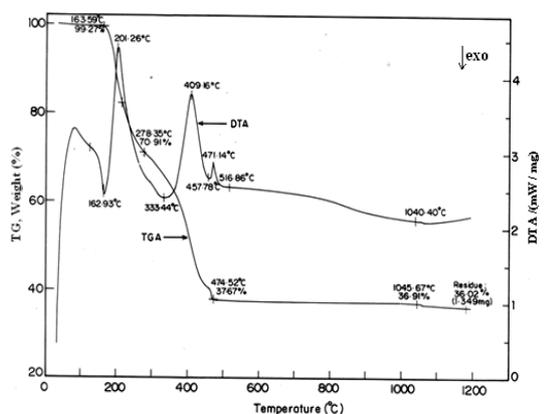
Fig. 3.4 TG-DTA thermogram of ZGuP and GCC
