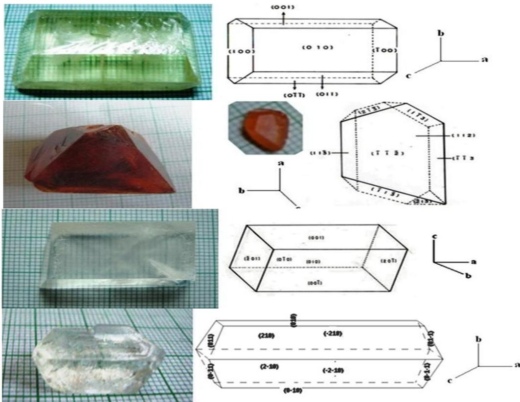
Fig. 1.1(b) Bulk crystals of Gu-3NB, GPA, ZGuP and GCC grown by slow cooling technique with Morphology.
