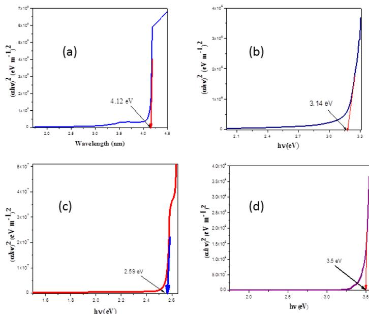
Figure 5. Tauc's plot of a) 2ADPTS b) 2,6DPT c) ISPA d) 2APD
