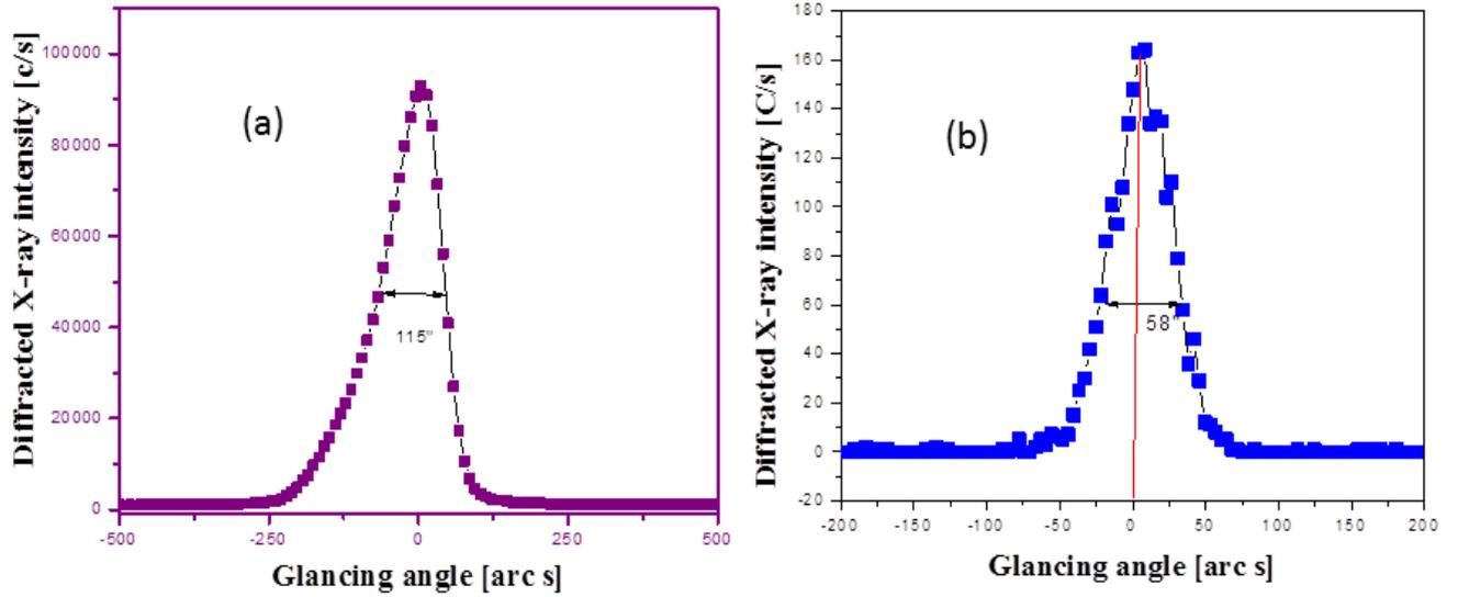
Figure 6. HRXRD curves of (a) 2ADPTS and (b) 2,6DPT crystals
