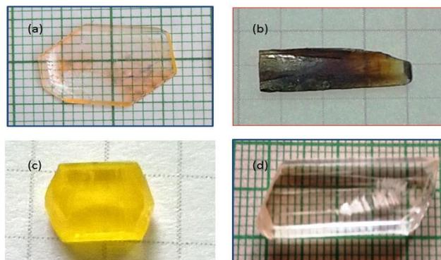
Figure 2. (a) As grown 2ADPTS crystal, (b) As grown 2,6DPT crystal, (c) As grown ISPA crystal, (d) As grown 2APD crystal
