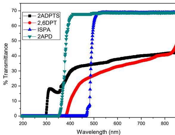
Figure 4. Optical transmittance spectra of the grown crystals
