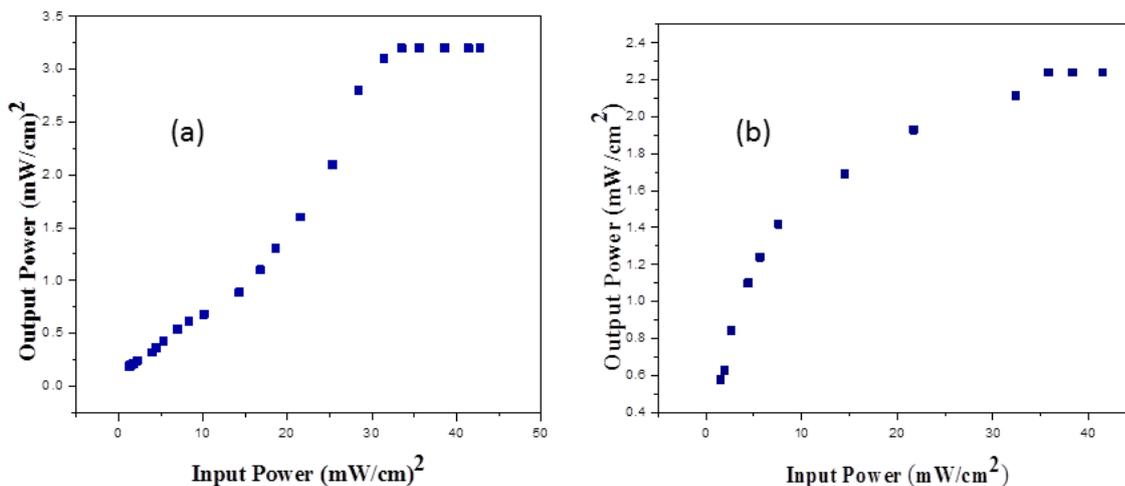
Figure 9. Optical limiting curves of (a) ISPA and (b) 2APD crystals
