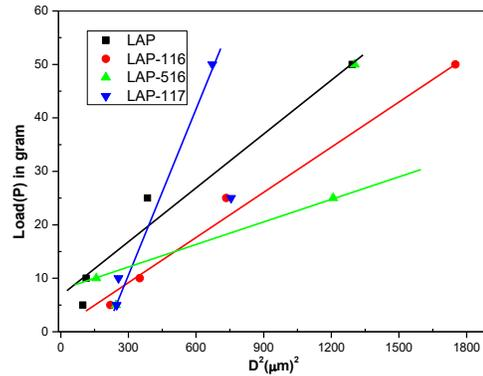
Fig.6a: Variation in the load  $P$  (grams) with  $d^2(mm^2)$ .
