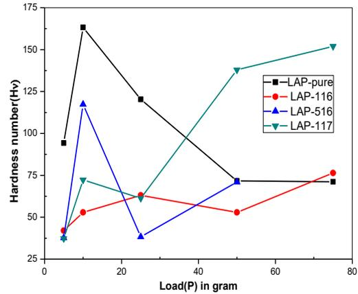
Fig.6: Variation in the Vickers hardness  $H_v$  with load  $P$  (grams).
