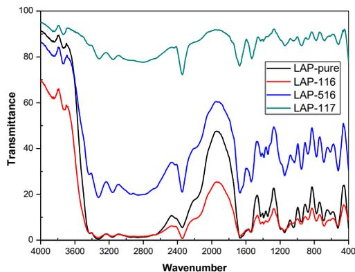
Fig.3: FTIR spectrum of pure and irradiated single crystal
