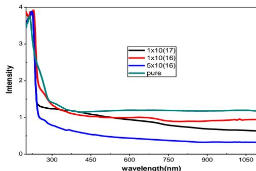
Fig.4: Plot of Absorbance vs. wavelength (nm) for pure and irradiated LAP single crystal
