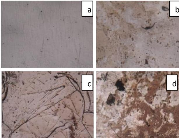
Fig.7: Micrograph of pure LAP and irradiated single crystals (a: pure, b:  $1 \times 10^{16}$  c:  $5 \times 10^{16}$ , d:  $1 \times 10^{17}$ ).
