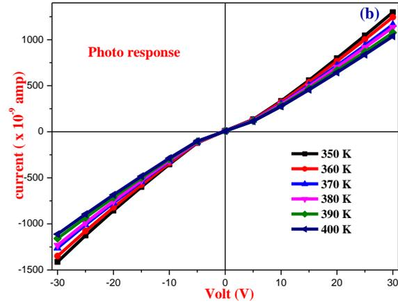
Fig. 6 (a) Variation of dark current versus applied voltage with temperature and 6(b) Variation of photocurrent versus applied voltage with temperature under illumination.
