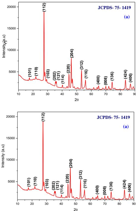
Fig. 2 (a) Powder X-ray diffraction pattern of the CdGa<sub>2</sub>Se<sub>4</sub> polycrystalline material and (b). Powder X-ray diffraction pattern of the grown single crystal wafer cut along the growth direction
