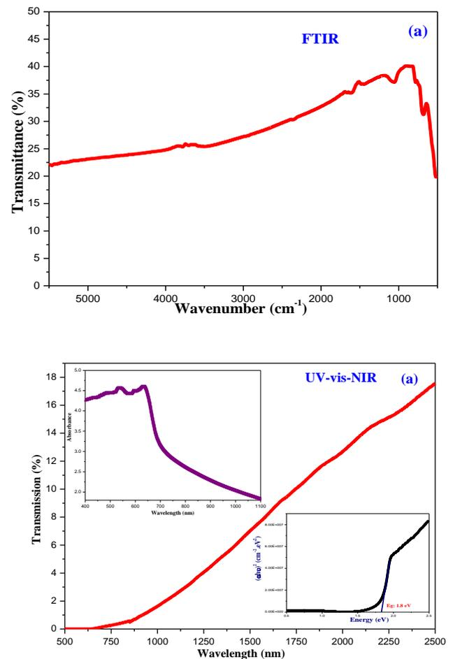
Fig. 5 (a). UV-vis-NIR transmittance, upper inset absorption spectra and bottom inset Tauc plot and (b) FTIR transmittance spectra of  $\text{CdGa}_2\text{Se}_4$  crystal.
