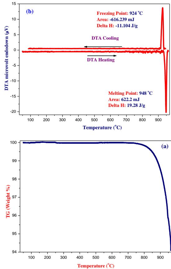
Fig.3 (a) TG and (b) DTA analysis of CdGa<sub>2</sub>Se<sub>4</sub> single crystal
