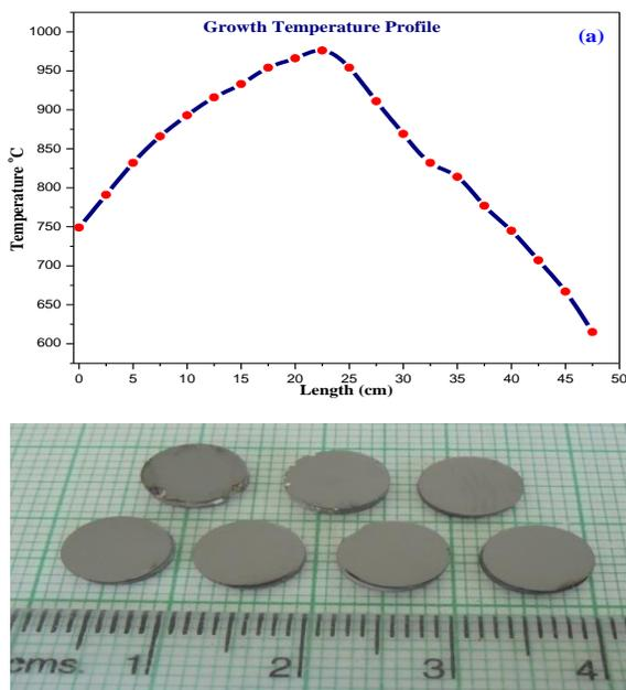
Fig. 1 (a) Temperature profile for growth furnace and (b) Cut and polished CdGa<sub>2</sub>Se<sub>4</sub> single crystal wafers
