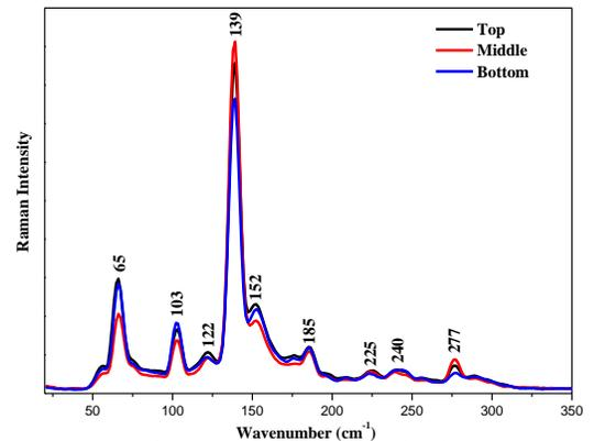
Fig. 4. Raman spectra of grown CdGa<sub>2</sub>Se<sub>4</sub> single crystal at different parts
